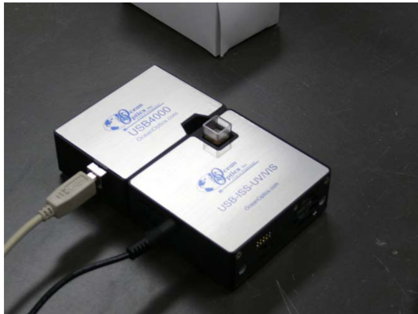
Figure 4.5. Portable UV-Vis Spectrophotometer Used to Estimate SOC in Soil.
