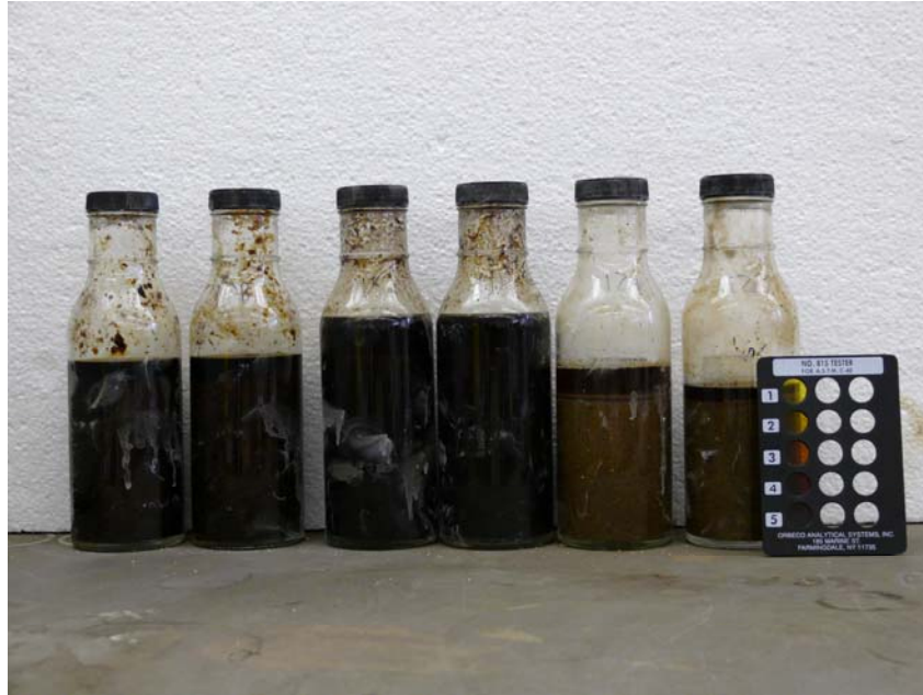
Figure 3.2. Samples with 1, 3, and 0.5 Percent Compost after TEX-408-A Test.
