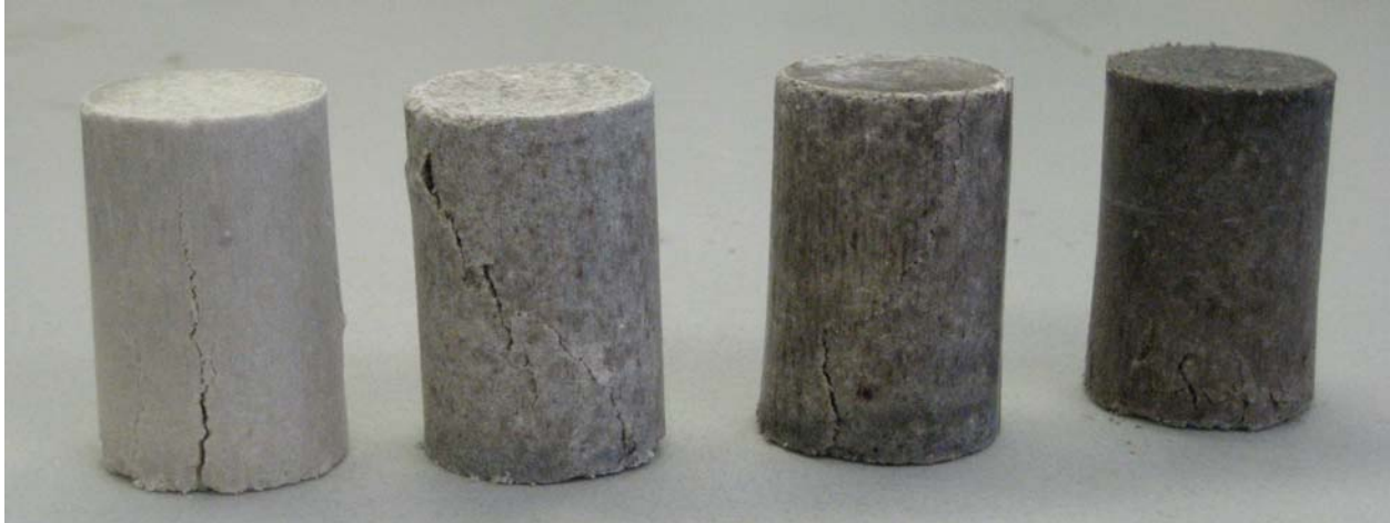
Figure 5.8. Harvard Miniature Samples of Sand, Smectite, Lime, and Different Contents of HA Ranging from (left to right) 0, 0.5, 2.0, and 5.0 Percent.
