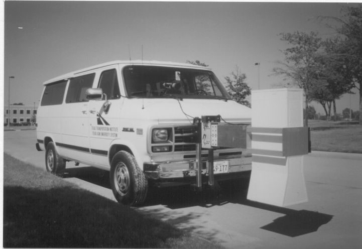
(a) TTI GPR Equipment
