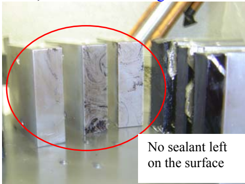
a) Typical adhesive failure
