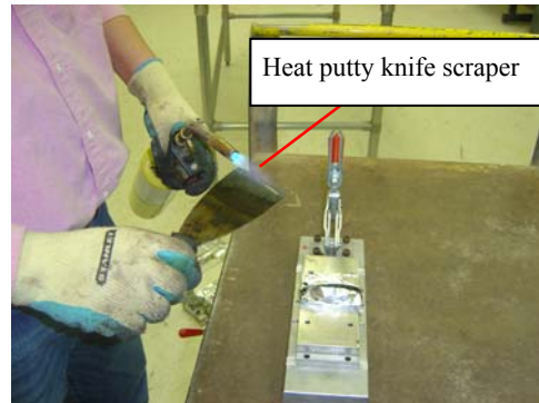
b) Heat the putty knife scraper
