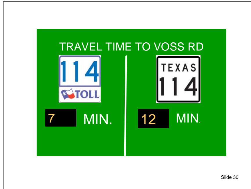
Figure 37. Focus Group Slide 30 Showing the Comparative Travel Time Sign Developed by the Researchers.
