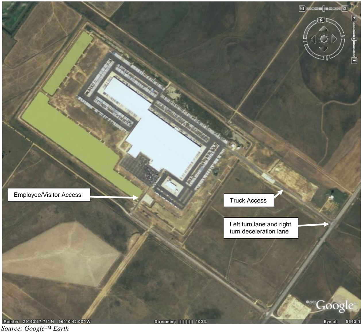
Figure C-1. Aerial Photograph of DC with Separate Inbound and Outbound Access. One driveway each for truck and employee/visitor access; driveways well separated from nearest intersection. Truck driveway provides ample queuing space for inbound and outbound trucks to check in at security booth. Employee/visitor driveway provides queuing length for outbound vehicles during shift changes.
