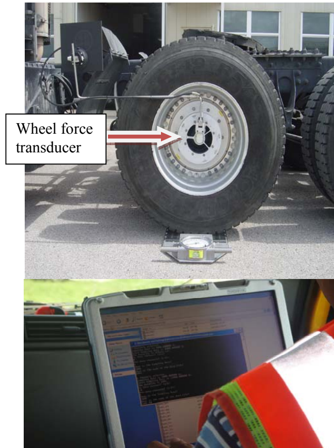
Figure 24. Comparison of Wheel Force Transducer with Static Scale.
