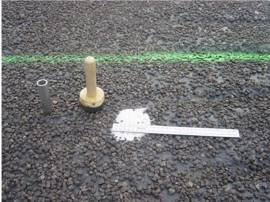
Figure 32. Sand Patch Test Conducted.
