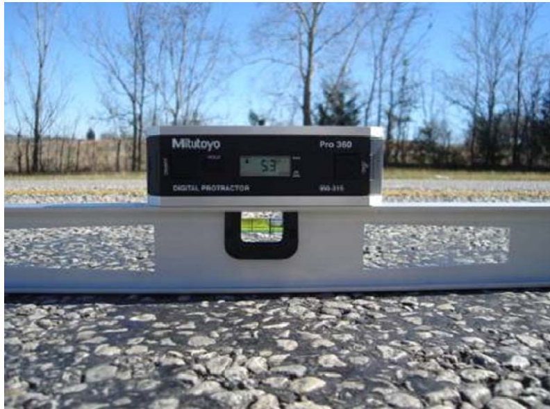
Figure 22. Slope Measurement Using a Digital Protractor.
