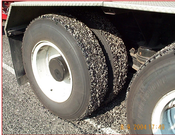
Figure 1. Seal Coat Damage due to SHL Moves.
