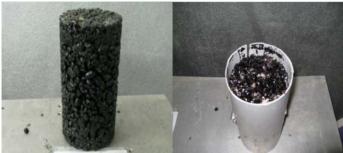
Figure 16. Molded Seal Coat Mixture.
