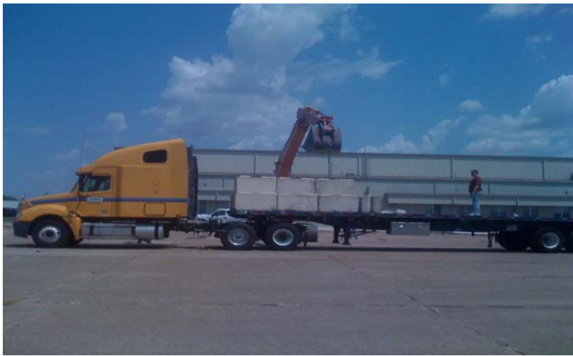
Figure 35. Test Truck for Bryan District Tests.
