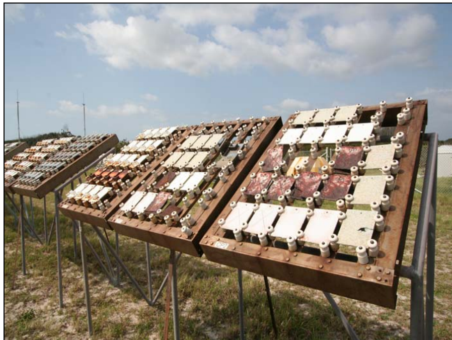
Figure 20. Test Panels Exhibiting Corrosion.
