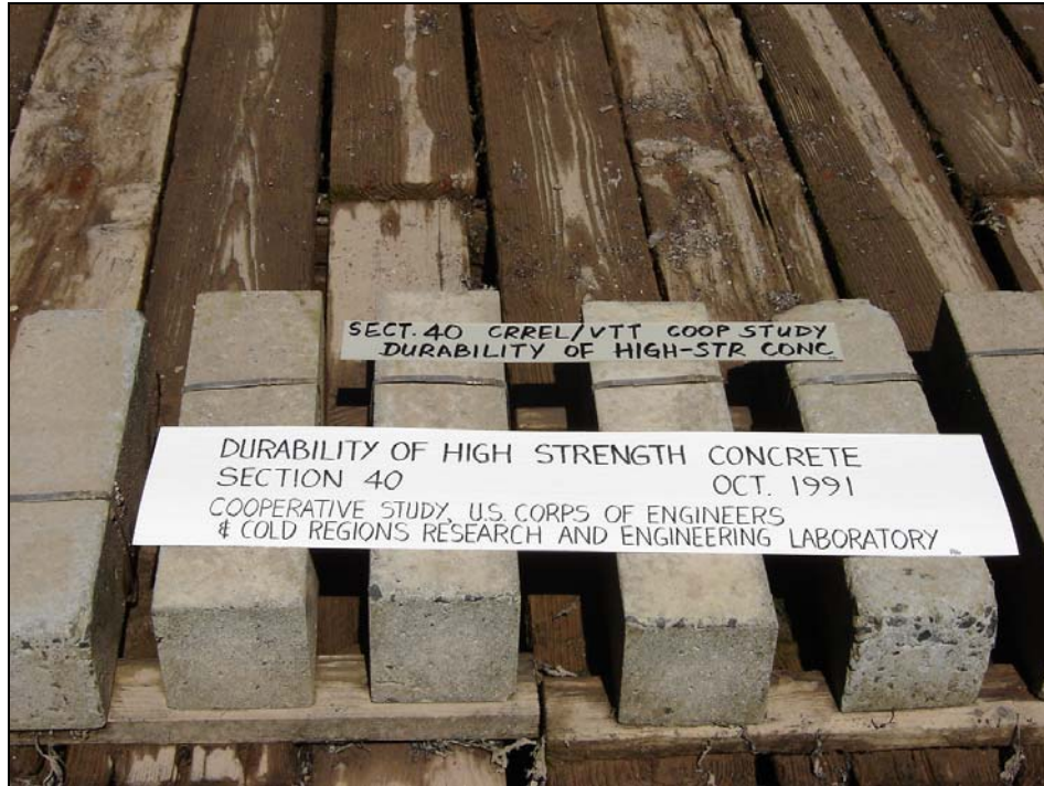
Figure 28. Durability Test of High-Strength Concrete.
