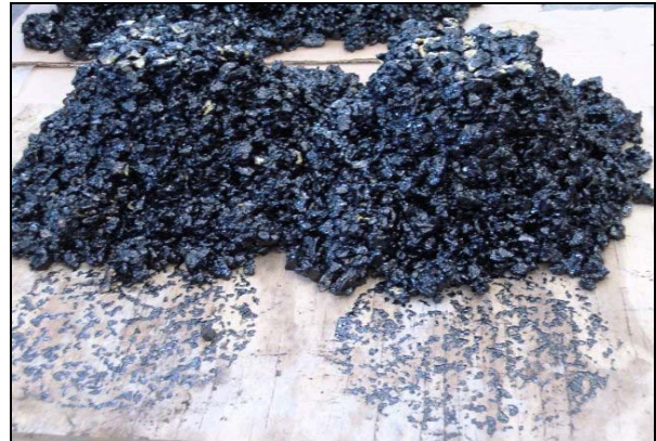
Figure 39. (a) Effect of Compaction Energy on Cantabro Loss and (b) US-290-AR Mixture Failure at High Temperature (140°F [60°C]).
