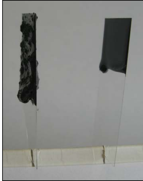
Figure 27. Asphalt Rubber Slides Prepared with Original Asphalt Rubber (Left) and Asphalt Rubber Filtered on Sieve 80 (Right).
