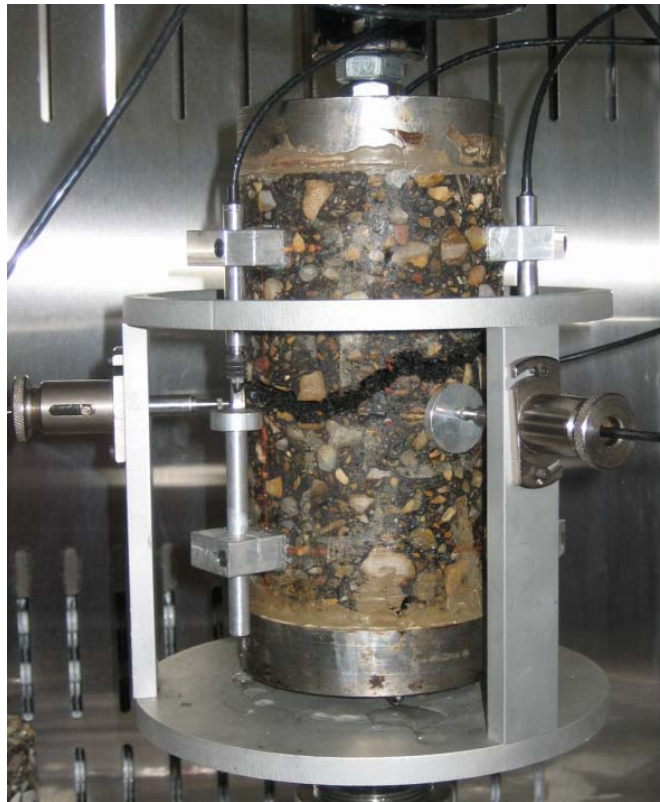
Figure 3-8. Test Sample after Failure inside the MTS.
