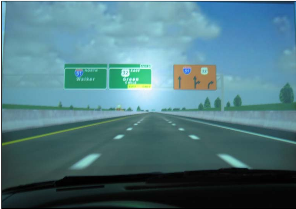
Figure 17. Misaligned Guide Signs with No Arrows and Temporary Signs.
