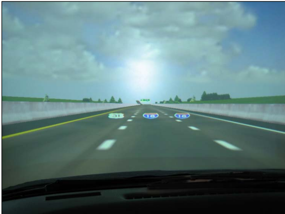
Figure 18. Route Shield Pavement Markings.
