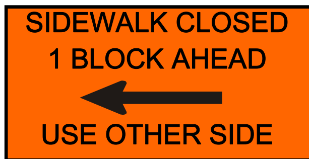
Figure 28. Recommended Advance Warning Sign.
