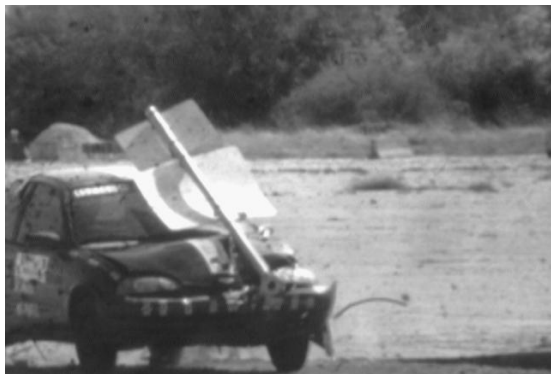
Figure C4. Sequential Photographs for Test 452108-4 (Oblique and Perpendicular Views).
