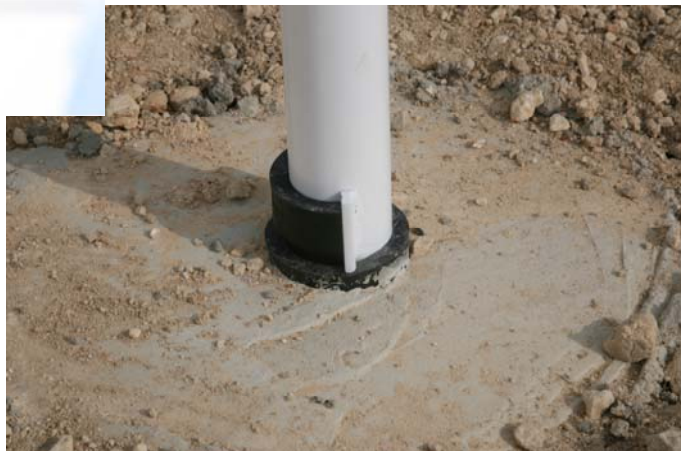
Figure 2. Shur-Tite® Multiple-Mailbox Mount before Testing.
