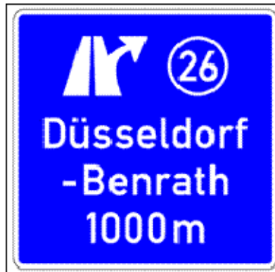
Figure 8. Autobahn Exit Announcement Sign.
