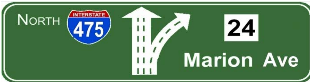
Figure 17b. Advance Guide Sign (Located approximately ½ mile in advance of exit and centered over the four approach lanes)
