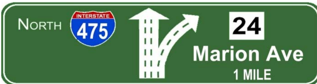
Figure 17c. Advance Guide Sign (Located 1 mile in advance of exit and centered over the four approach lanes)
