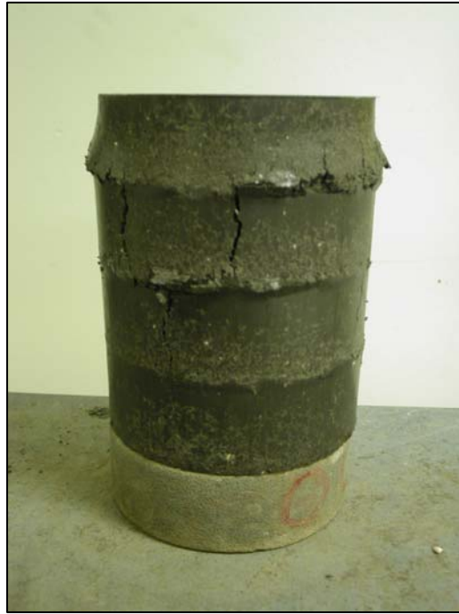
Figure 3.1. Soil Specimen after Triaxial Testing.
