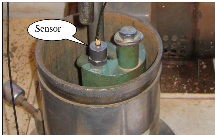
Figure 2.5. Accelerometer Attached to Top of Rainhart Impact Hammer.
