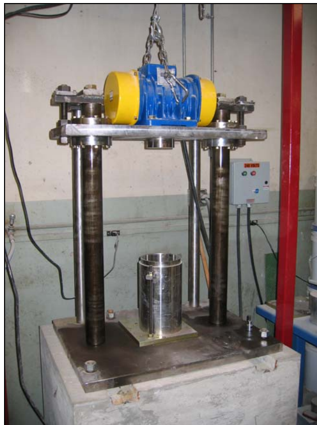
Figure 3.3. Prototype Lab Vibratory Compactor.
