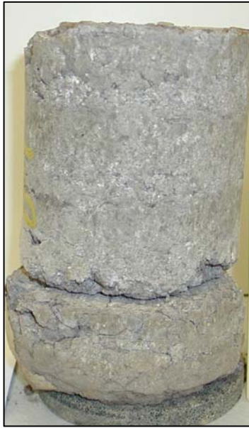
Figure 3.2. Layer Separation in Swell Test of Specimen Compacted in Lifts with Impact Hammer Compaction (Sebesta, et al. 2004).
