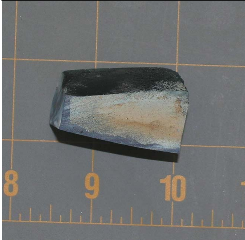
Figure 4.4. Partially Impregnated Compacted Sand Sample.
