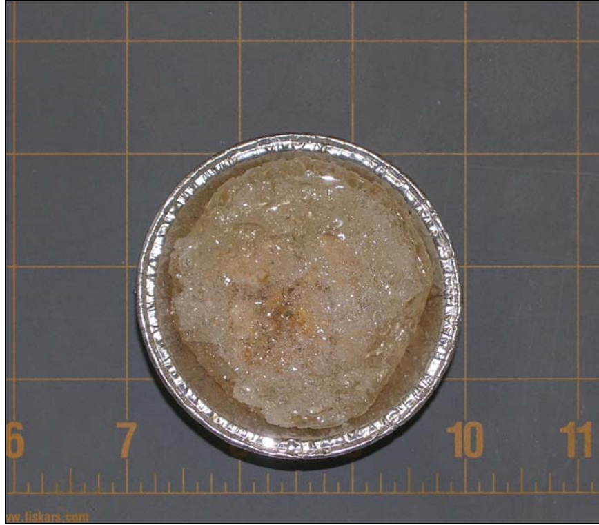
Figure 4.1. Sample Cured in a Vacuum Oven Using L R White Resin.
