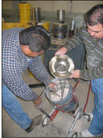
Figure 2.2. Mixing in Molding Water with a Mechanical Mixer.
