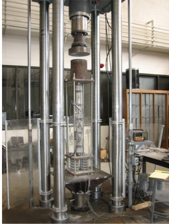
Figure 4.10. Loading with 500 kip (2220 kN) MTS Machine.
