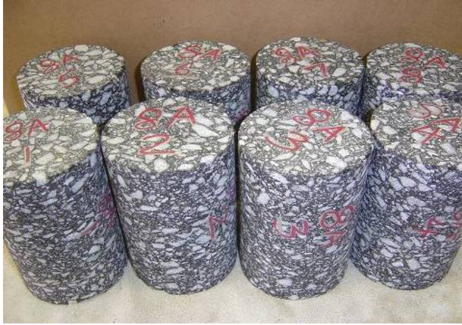
Figure 3-7. Examples of Prepared Specimens for Dynamic Modulus Test and Repeated Load Test.
