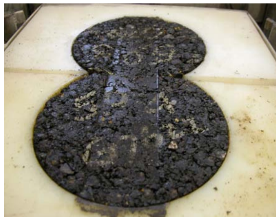
Figure 16. Trimmed HWTT Specimens.
