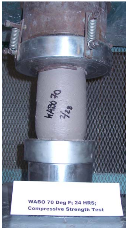
Figure 4.3 Compressive Strength Testing of Wabo ElastoPatch During and After Test
