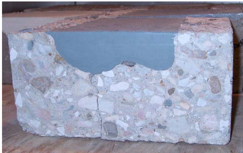
Figure 4.10 Spall after Thermo Cycling
