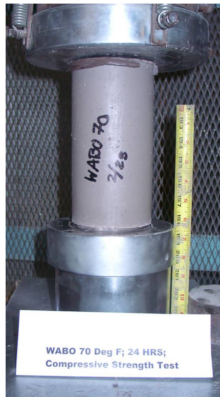
Figure 4.3 Compressive Strength Testing of Wabo ElastoPatch During and After Test
