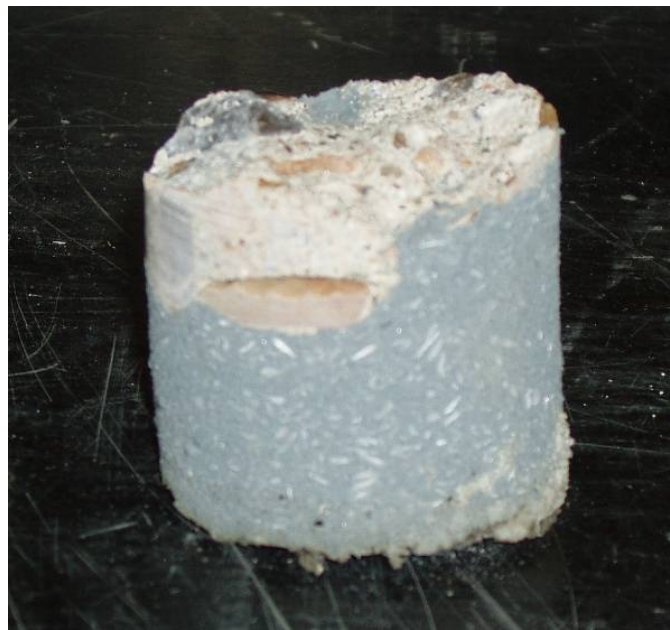
Figure 5.18 Delpatch Tested Tensile Bond Specimen
