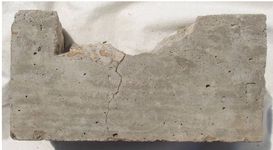
Figure 4.9 Photo of Simulated Spall
