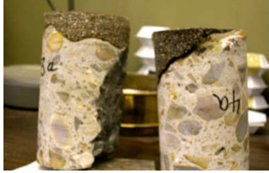
Figure 5.6 Cores Showing Broken Bond
