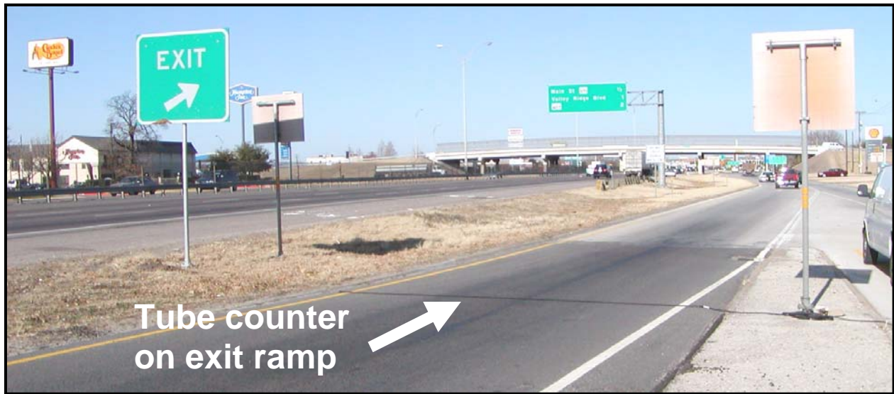
Figure 5-2. Collection of Exit Ramp Volume Using Pneumatic Tube Counter.
