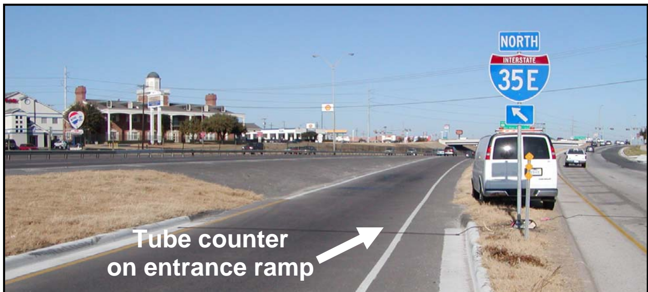
Figure 5-3. Collection of Entrance Ramp Volume Using Pneumatic Tube Counter.
