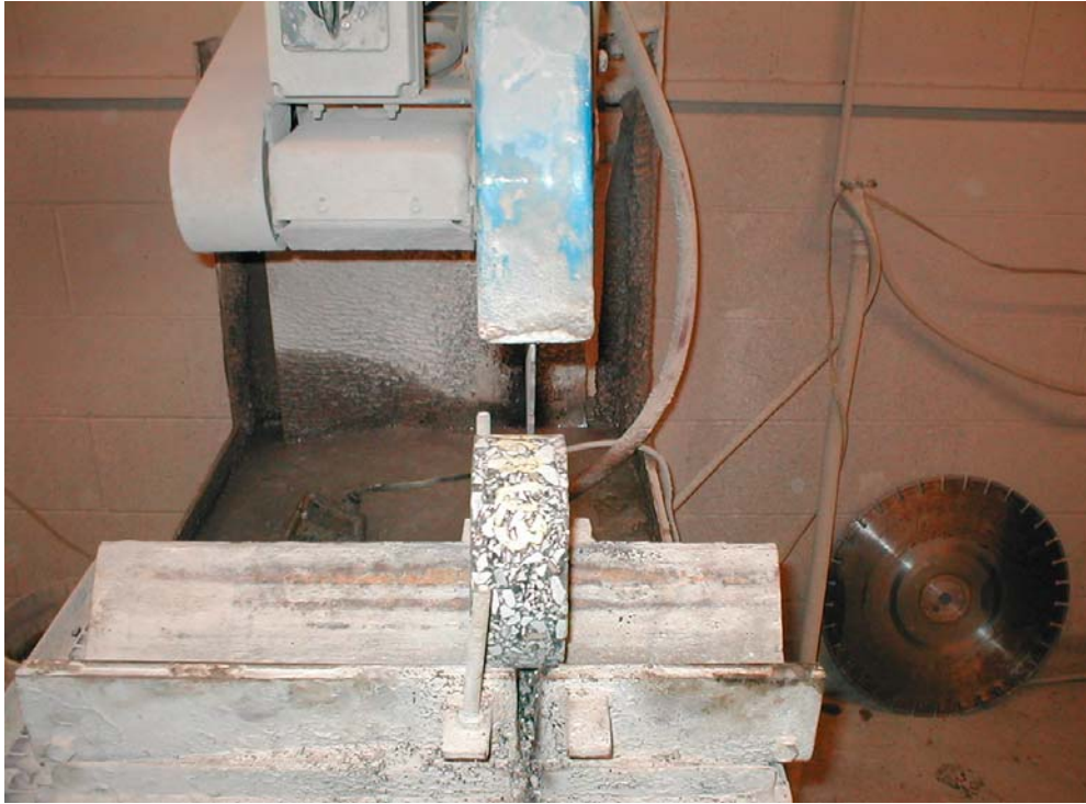
Figure 2-7. Slicing Cores for Further Testing.
