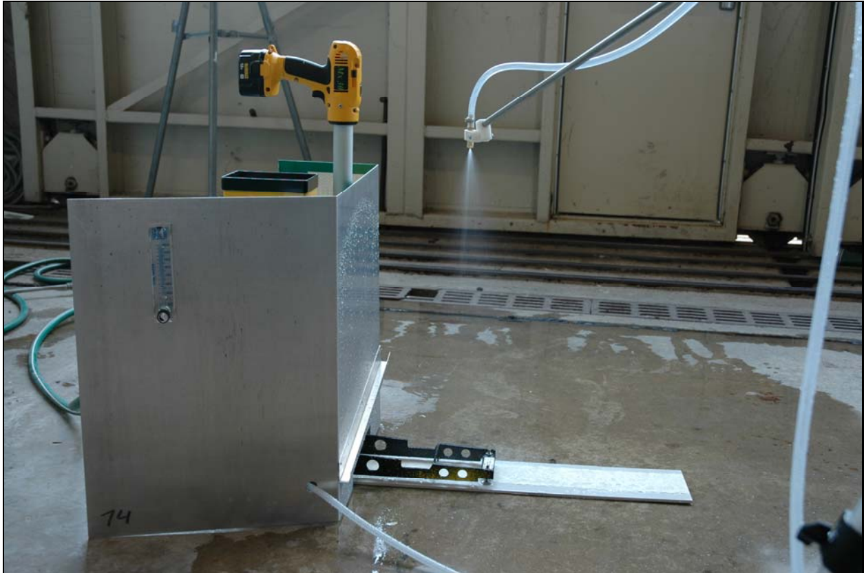
Figure 6. Continuous Wetting Setup for Spray Conditions (Rain > 1 in/hr).
