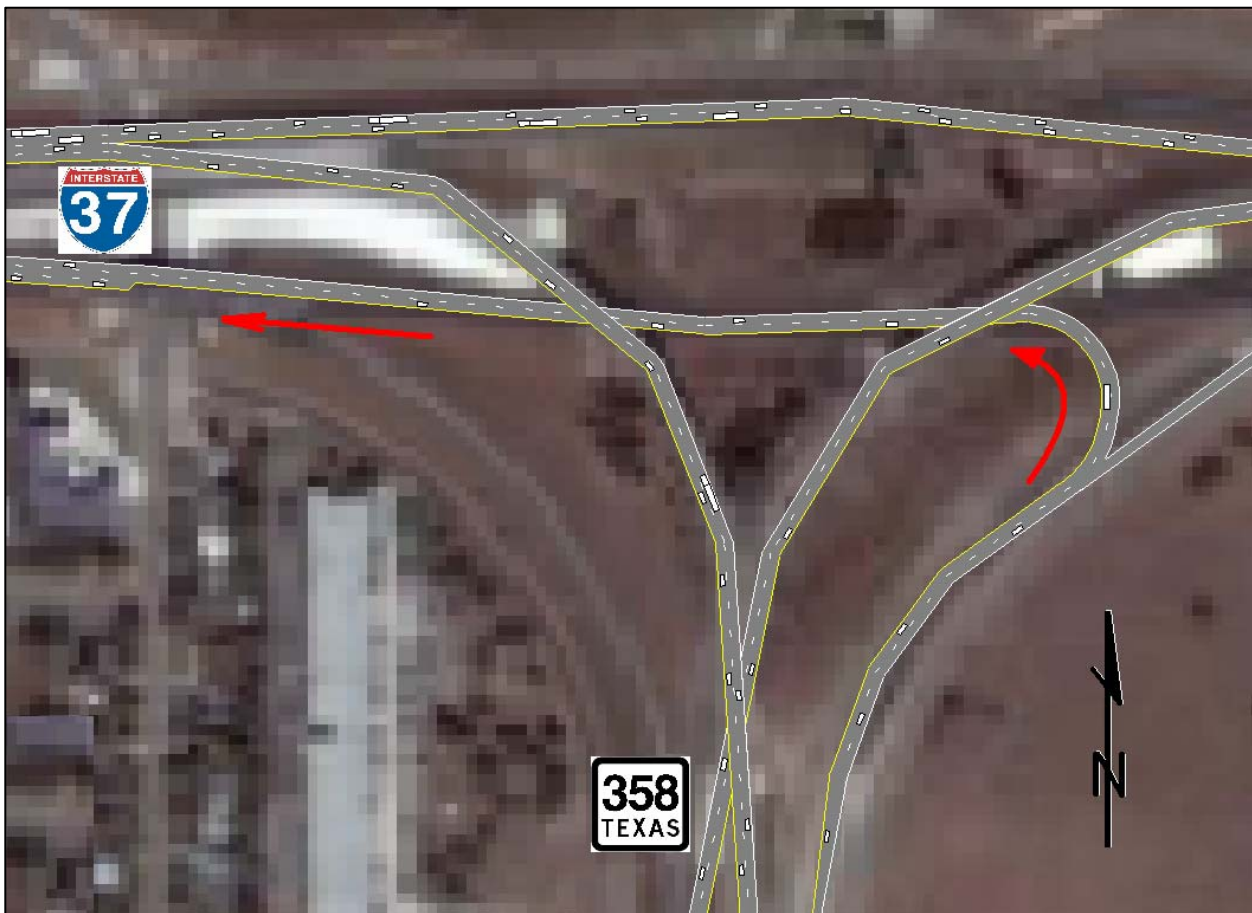
Figure 11-8. Special Contraflow Ramp from SH 358 onto I-37.
