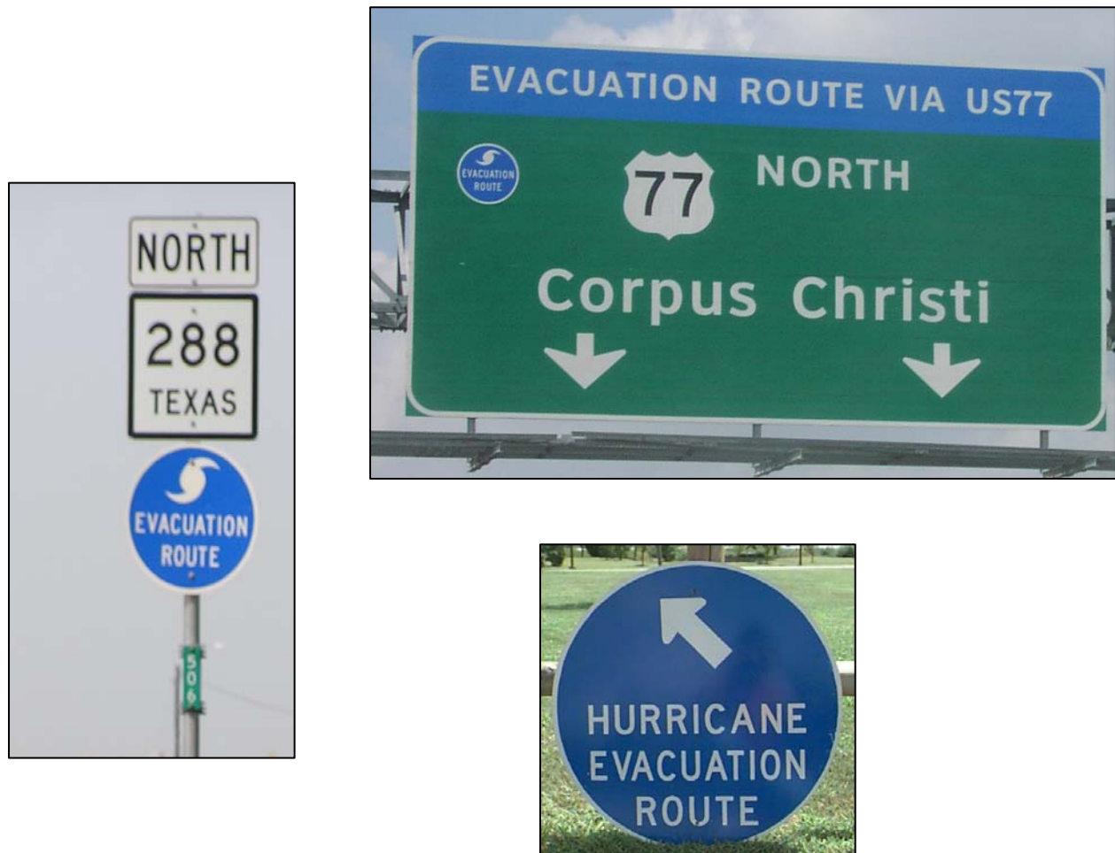
Figure 2-3. Alternative Formats for Evacuation Route Signing.
