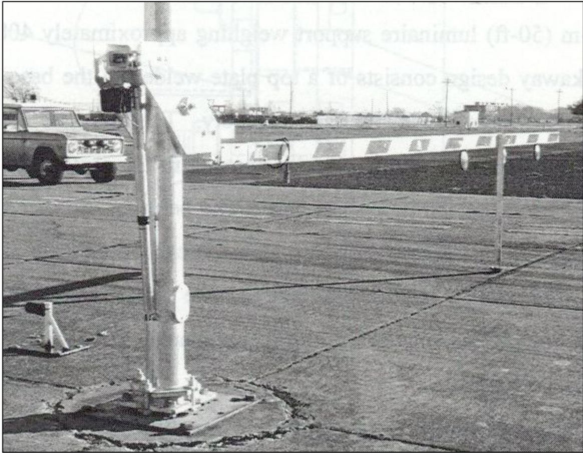
Figure 9-7. Crash-Testing of Wyoming's Road Closure Gate (33).
