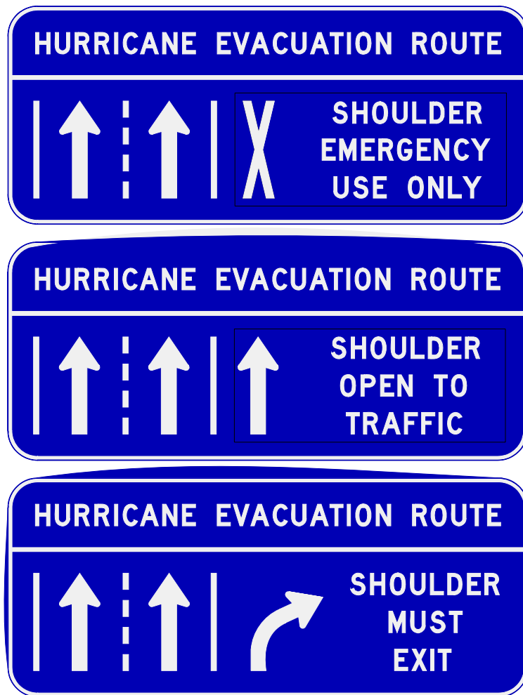
Figure 2-4. Signing for Temporary Shoulder Use during Evacuations in Corpus Christi.
