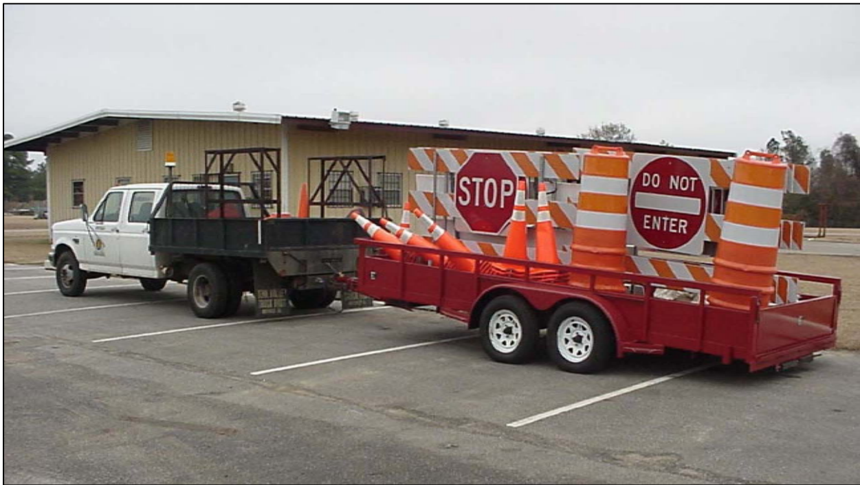
Figure 9-9. Dedicated Traffic Control Equipment (35).
