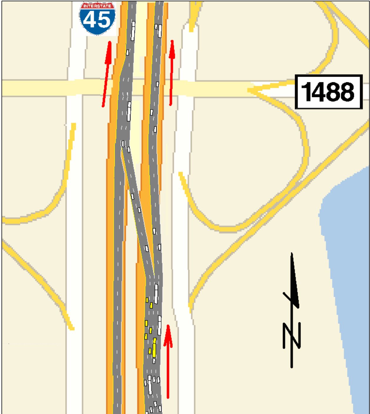
Figure 11-10. I-45 Contraflow Input from FM 1488 in Shenandoah, Texas.
