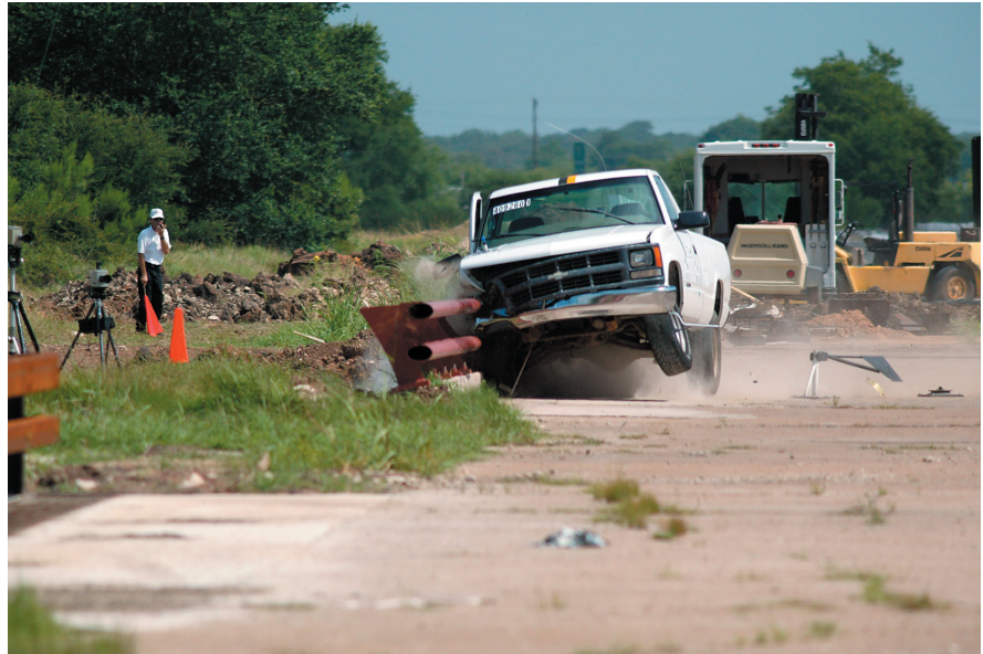
Successful Pickup Truck Test with T77 Bridge Rail.
