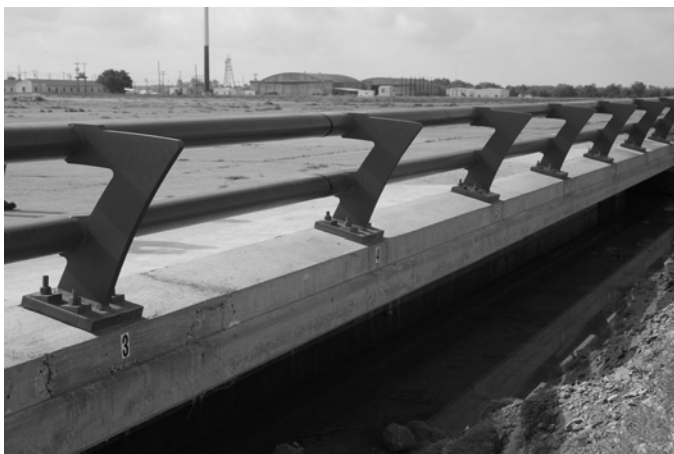
Figure 7. Modified T77 Bridge Rail Before Test 409260-1.
