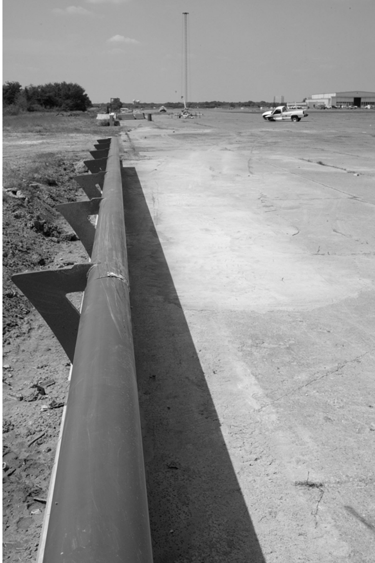
Figure 10. After Impact Trajectory Path for Test 448523-1.
