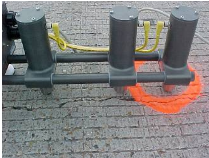
Figure 5.8. Example of PSPA Testing around a Core Location Following Proposed Field Test Protocol.
