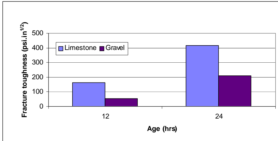
Figure 3.3. Fracture Toughness of Concretes at Different Ages.
