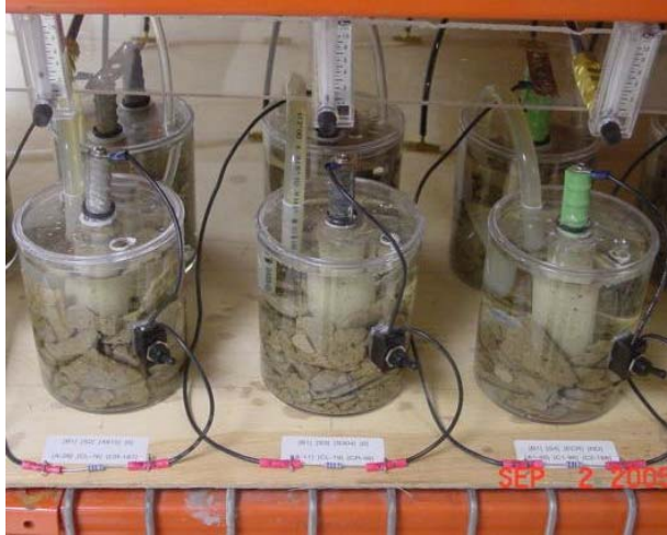
Figure 5. Rapid Macrocell Test Setup on the Rack.
