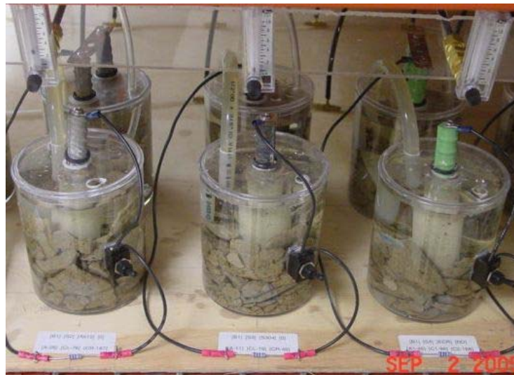
Figure III-15 Picture of Rapid Macrocell Test Setup on the Rack.
