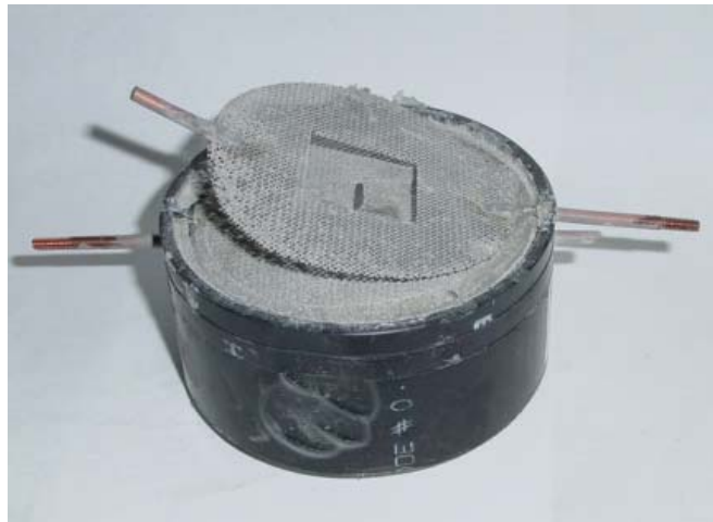
Figure A-3 Top Portion of the ACT Specimen with the Anode Mesh Disk Peeled Off.
