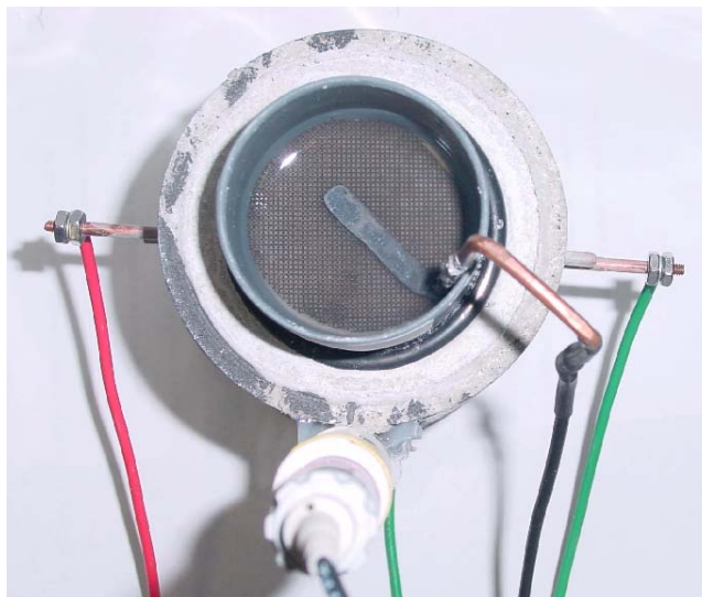
Figure A-11 Actual ACT Test Specimen Ready for Testing (Top View).
