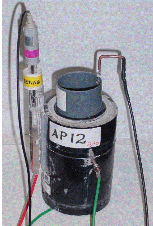
Figure A-10 Actual ACT Test Specimen Ready for Testing (Side View).
