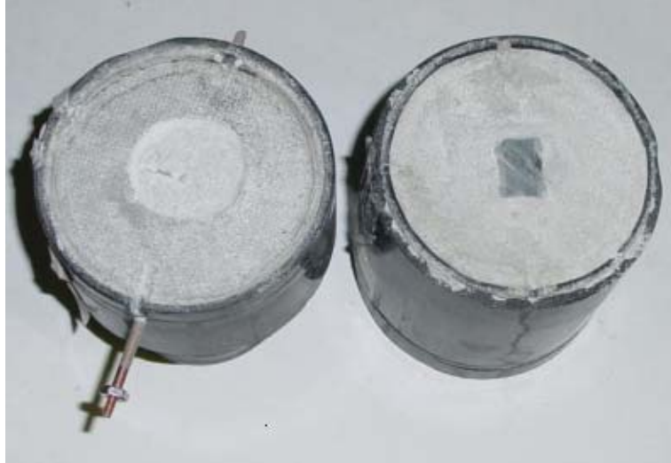
Figure A-4 Broken and Ground ACT Sample.
