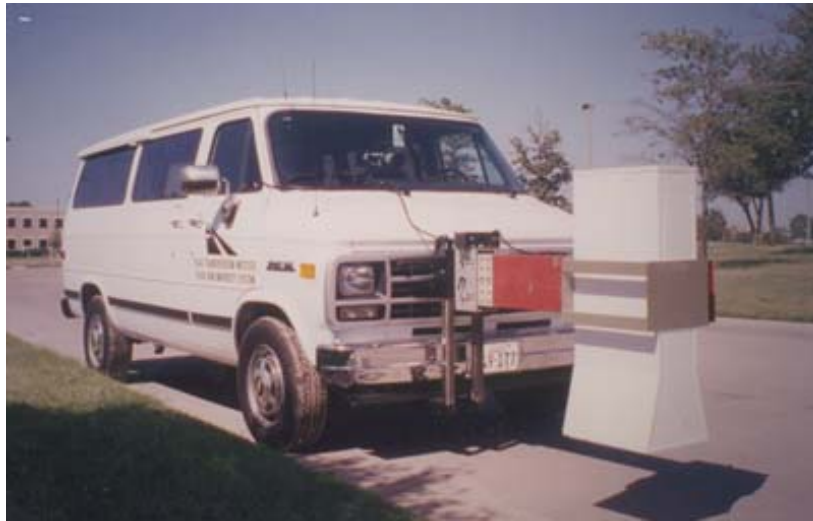
Figure 4-3. TTI's GPR System Setup.
