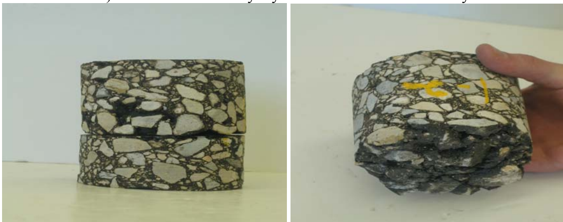
c) Cores from defect area
