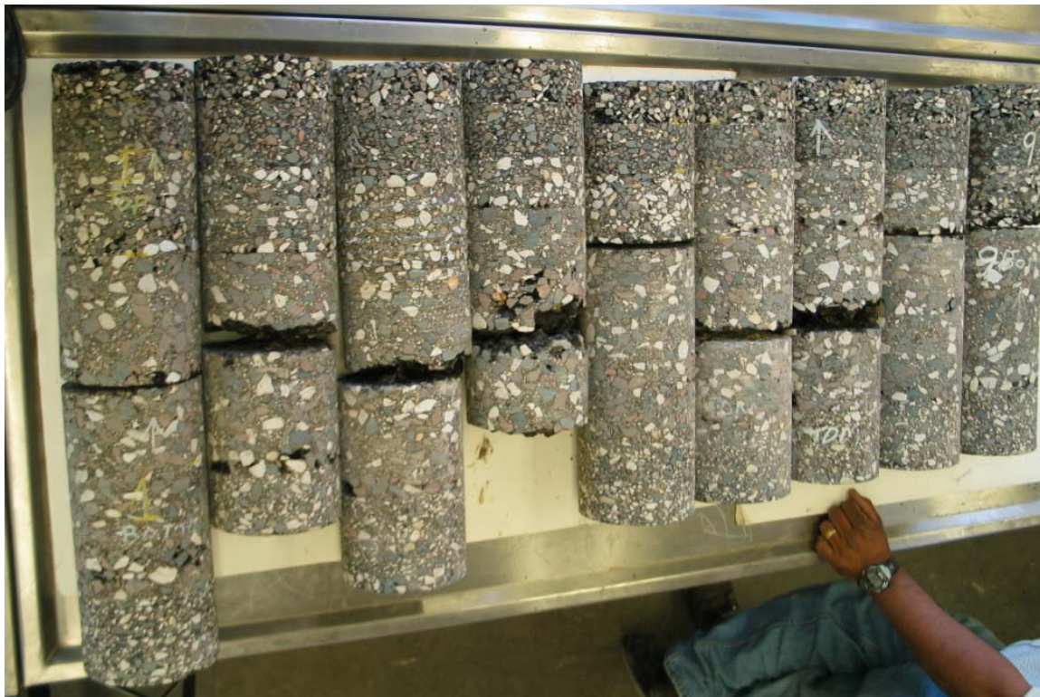
Figure 23. Cores Taken from the Zumwalt 2 Project in Laredo (Upper) and Young Brothers Project in Waco (Lower).
