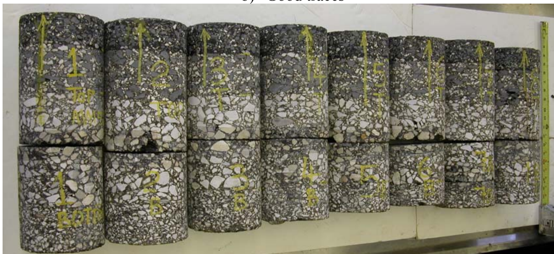
c) De-bonding of cores
