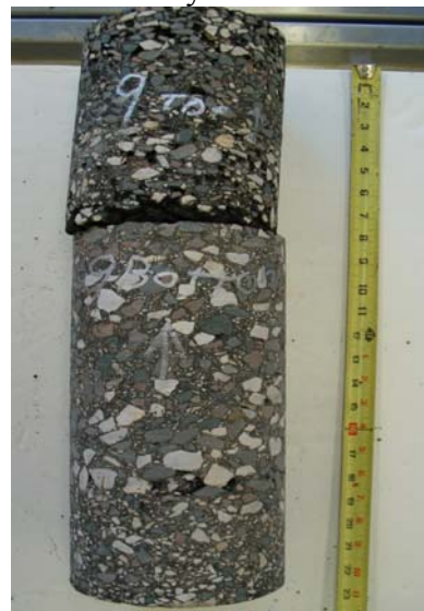
c) Core from defect location
