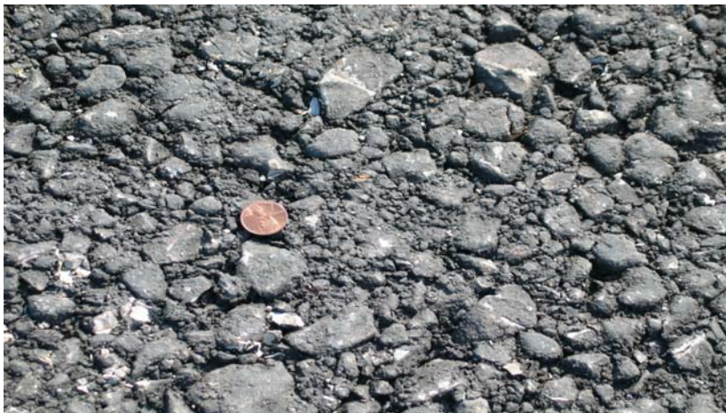
Figure 25. Coarse Texture of the 1-Inch SF Mix Used in San Antonio.
