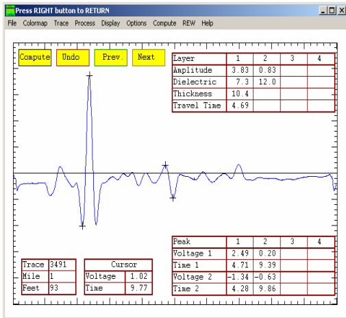
b) Low density at bottom of layer
