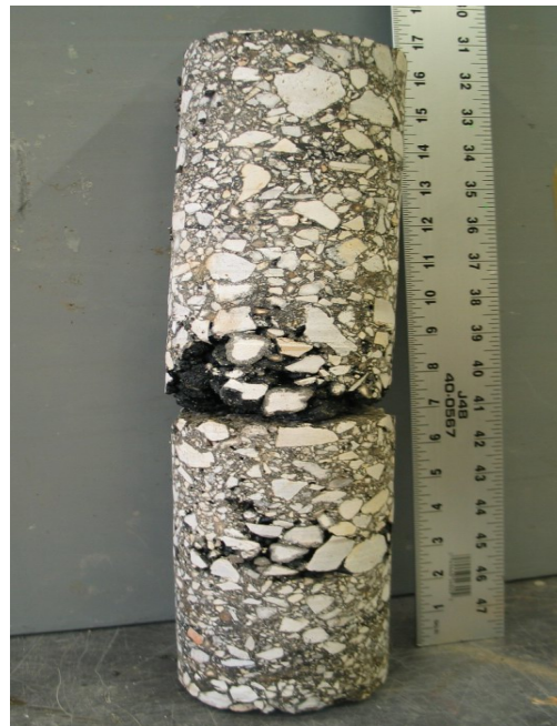
Figure 21. Severe Vertical Segregation in SF Layers.
