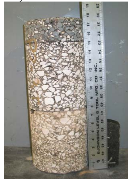
c) De-bonding in core
