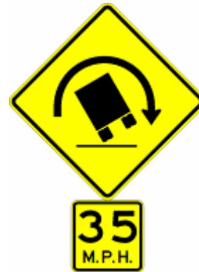
Figure 14. W1-13 – Standard Tipping-Truck Advisory Speed Warning Sign.
