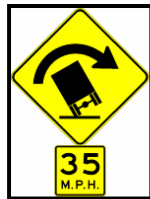
Figure 25. Modified Truck Advisory Speed Warning Sign (Houston).
