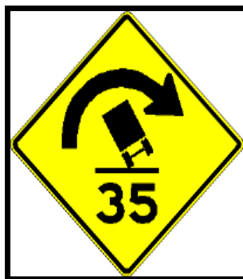
Figure 24. Modified Truck Advisory Speed Warning Sign.
