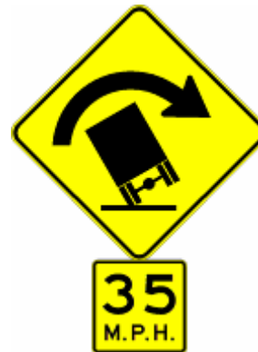
Figure 16. W1-13 – Truck Advisory Speed Warning Sign (Houston District).
