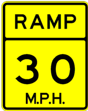
Figure 13. W13-3 – Ramp Advisory Speed Warning Sign.
