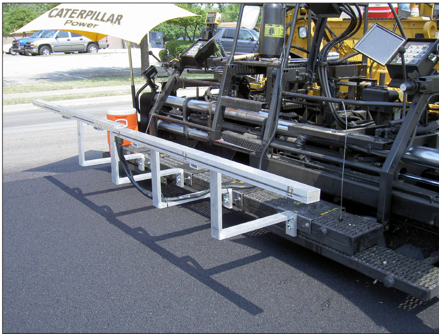
Figure 3. TTI's Pave-IR System Collecting Project Data.
