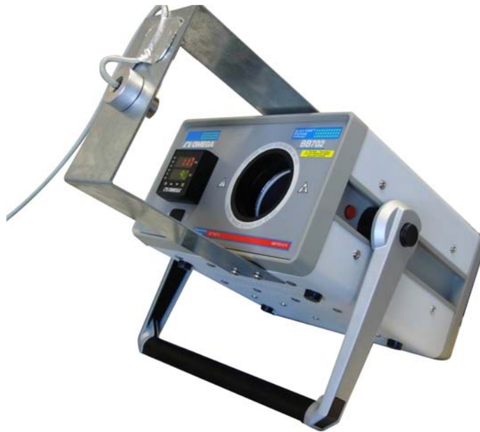
Figure 27. Infrared Sensor Installed in Blackbody Source for Calibration.
