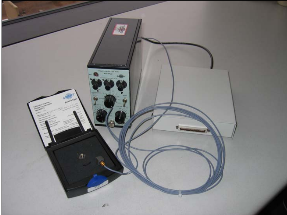
Figure 4.1. Accelerometer Instrumentation System for Vibratory Rollers.
