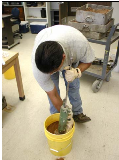
Figure 2.2. Tamping Mixed Soil in Preparation for Testing with Moisture Probes.
