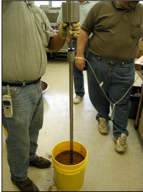
Figure 2.3. Installing Vertek Probe into Prepared Calibration Bucket.
