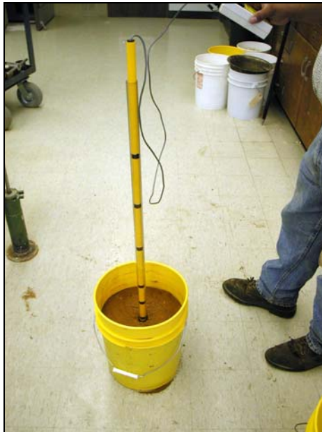
Figure 2.4. Collecting AquaPro Readings in Prepared Calibration Bucket.
