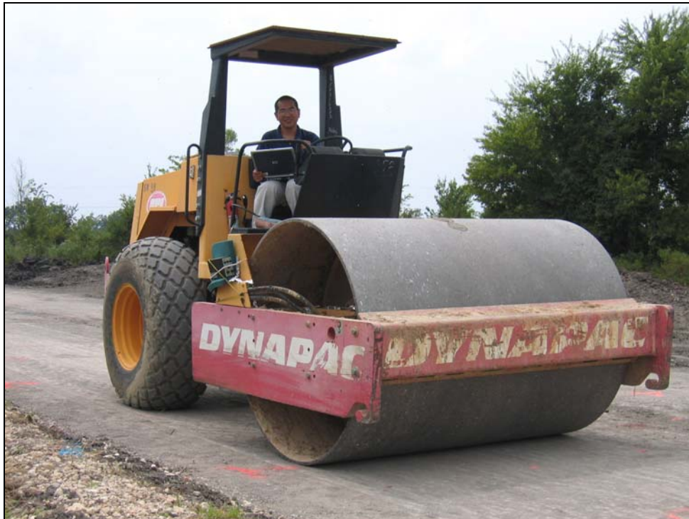
Figure 4.2. TTI Roller Instrumentation System in Operation on Construction Site.
