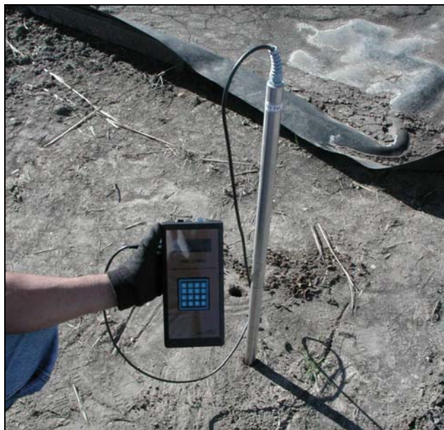
Figure 1.4. Adek Down Hole Dielectric Probe.
