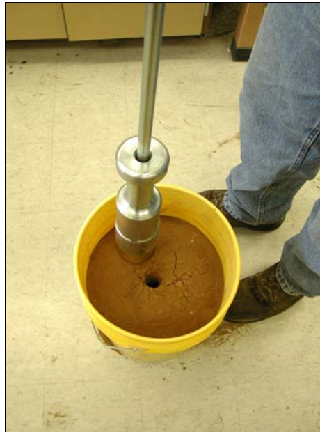
Figure 2.5. Collecting Control Sample from Soil Moisture Calibration Bucket.
