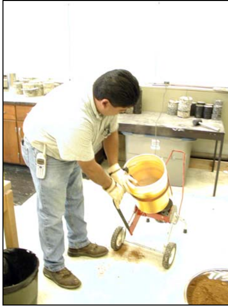
Figure 2.1. Mixing Soil for Laboratory Calibration of Moisture Probes.
