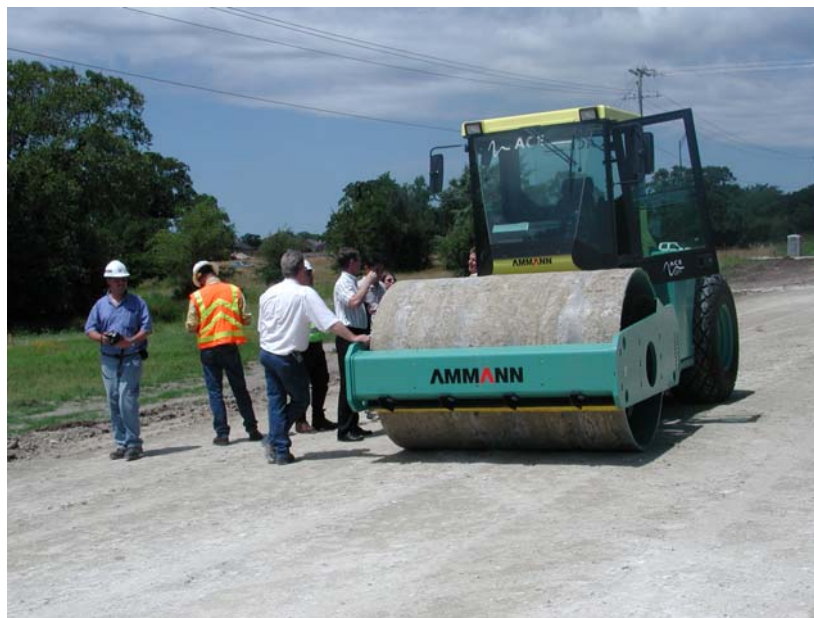
Figure 3.1. Ammann ACE-Equipped Vibratory Roller.
