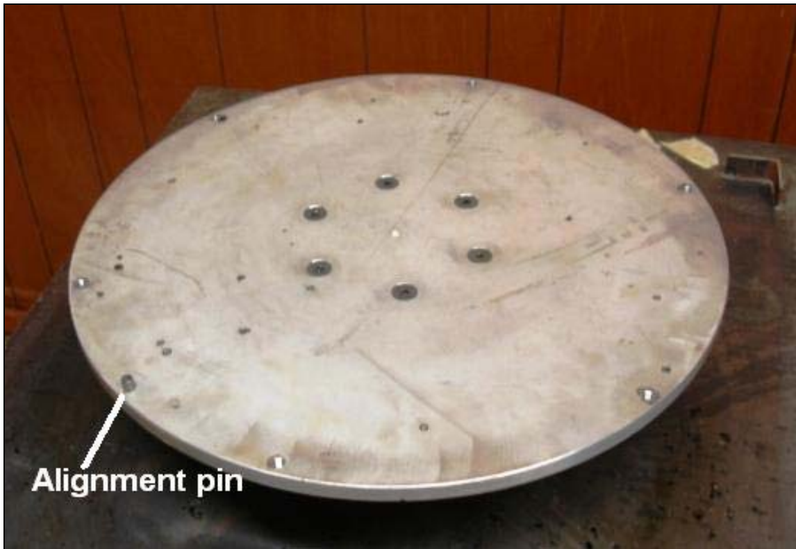
Figure 3.3. Alignment Pin Used to Position the Test Specimen on the Platter.
