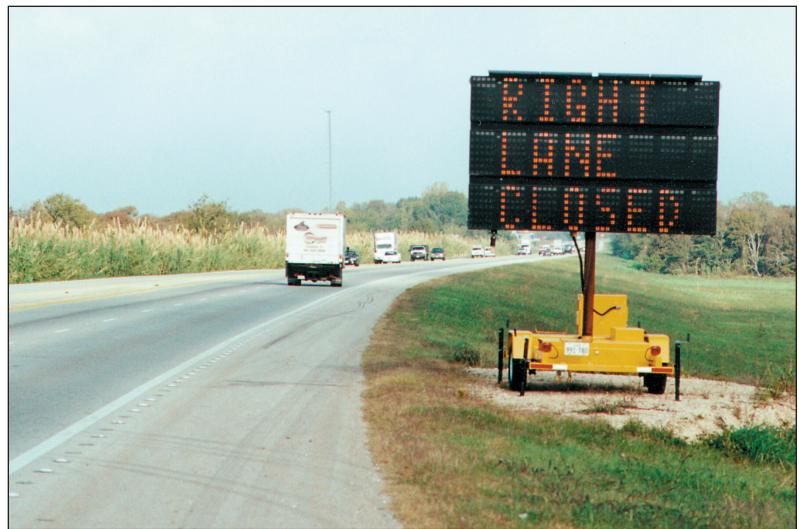
Figure 1. Work Zone Traffic Control Is Improved with Good PCMS Use.
