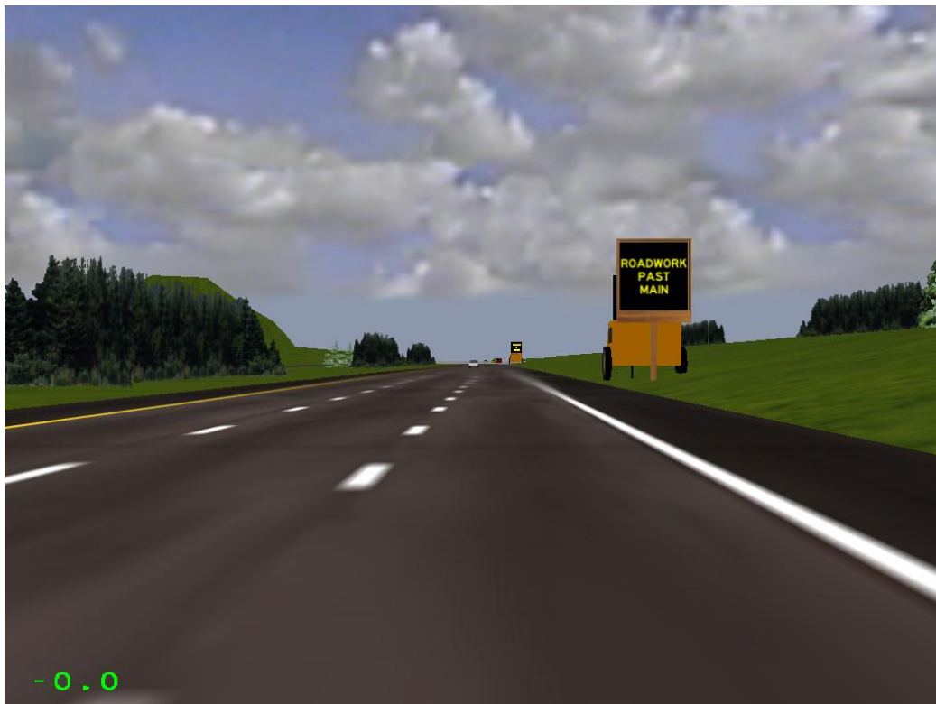
Figure 4. Representation of Sequential PCMS in the Driving World.
