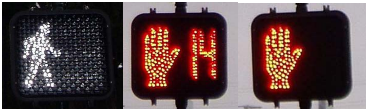
Figure 3-2. Displays in a Pedestrian Countdown Timer.
