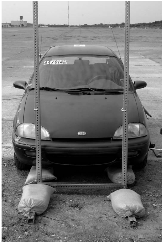
Figure 5-2. Vehicle and Support Geometrics before Test.
