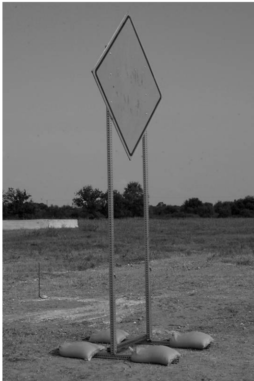
Figure 5-1. Sign Supports Used for Test.
