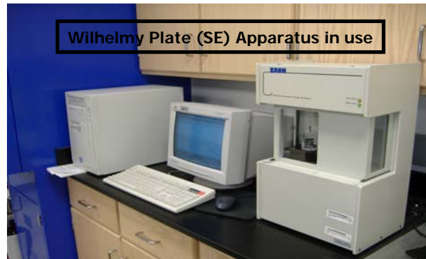
Figure 6-6. Wilhelmy Plate Test Setup.
