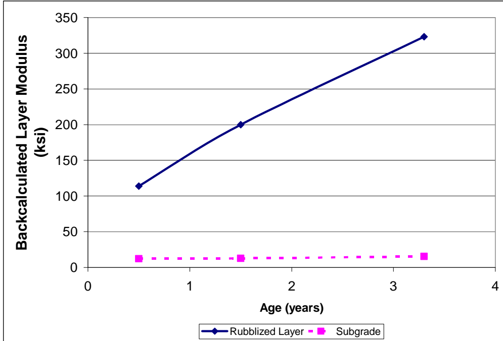
Figure 5.4. Average Pavement Layer Modulus with Time for US 83 from FM 3256.
