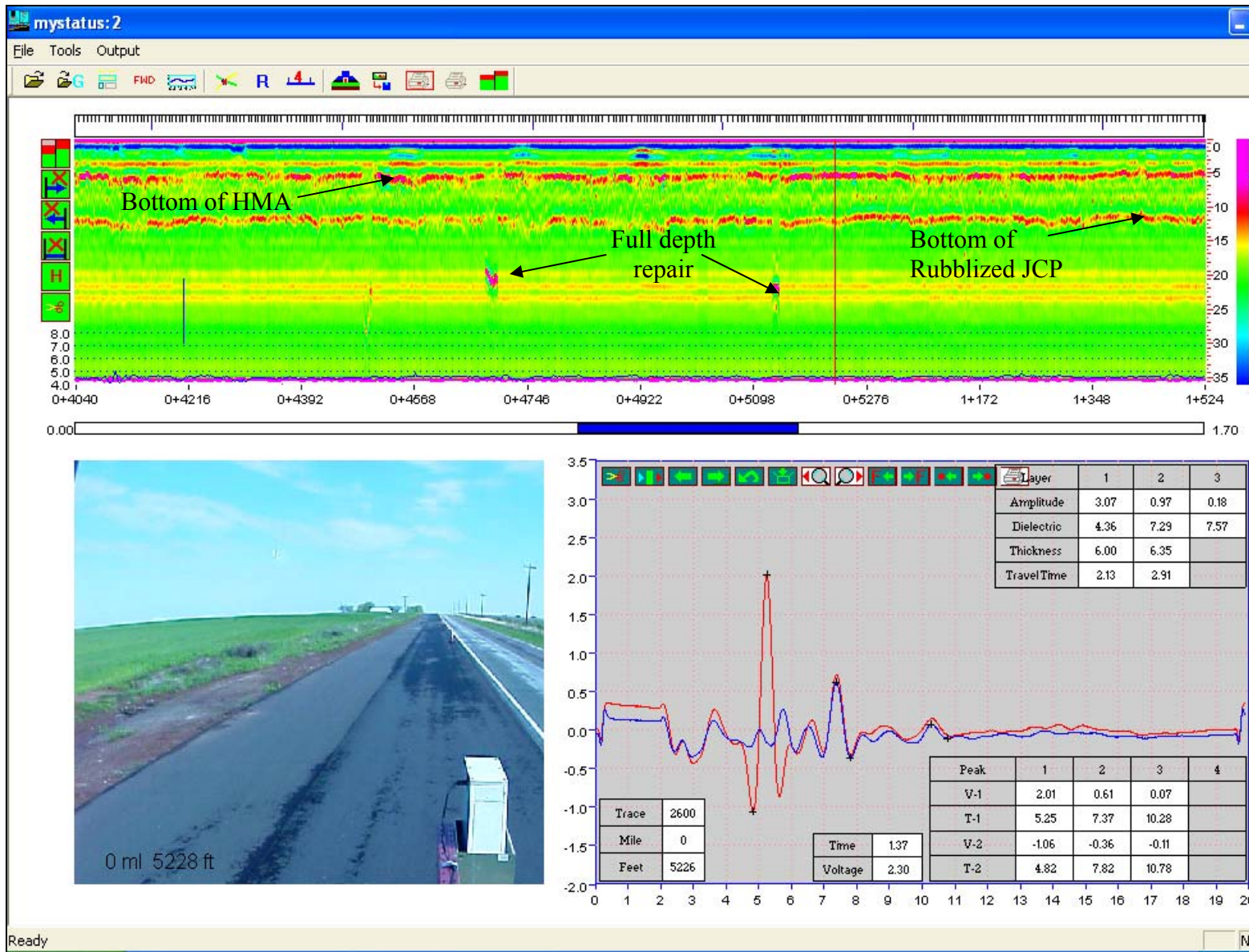
Figure 7.17. Example GPR on US 83 from King / Cottle County Line.
