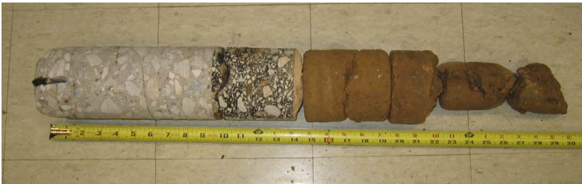
Figure 3.6. Core over Saw Cut on Loop 288. Note that the concrete did not crack at the sawcut.
