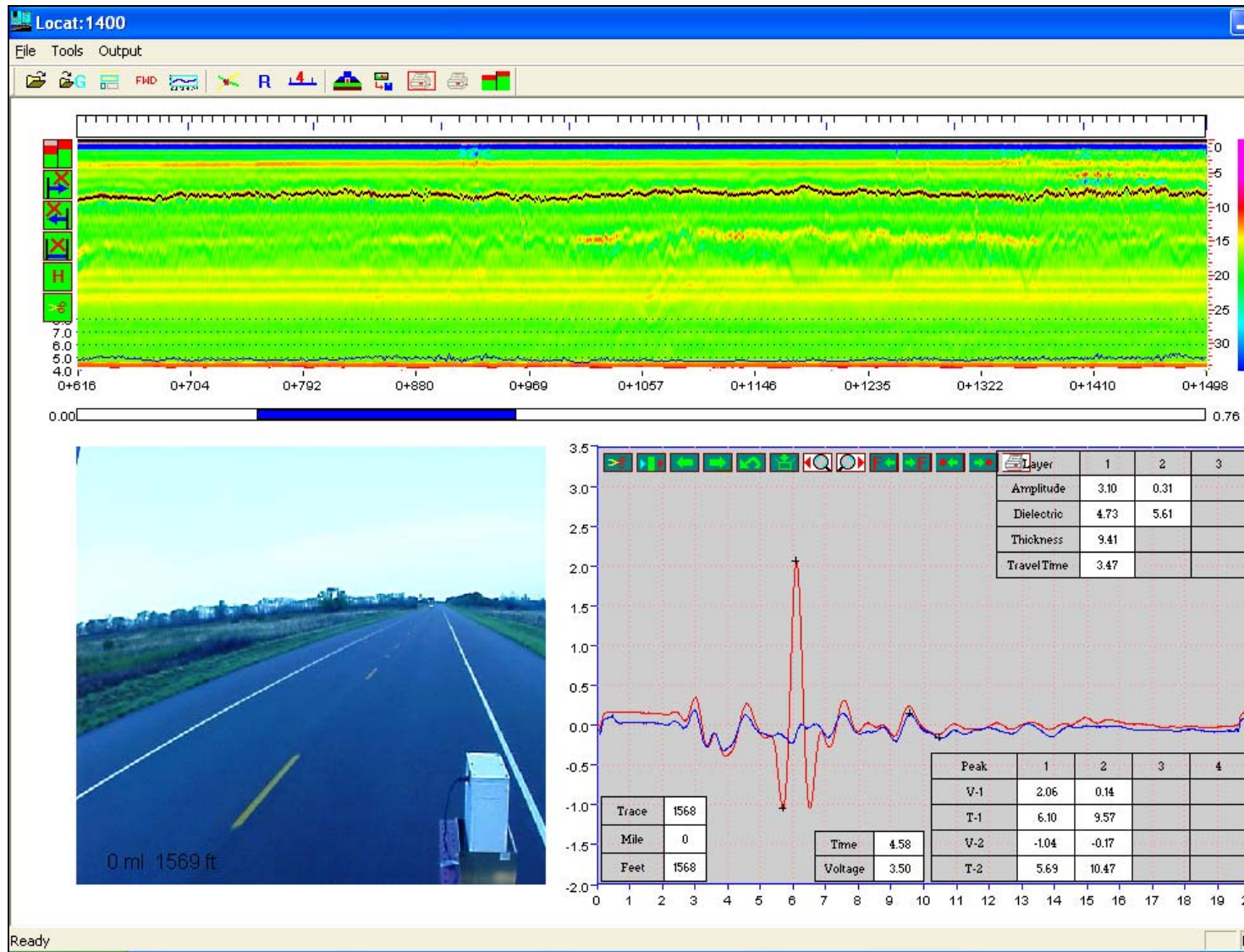
Figure 5.2 . Example GPR Data on US 83 from FM 3256. Note: black line in GPR pattern is top of rubble layer.
