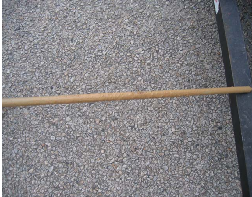
Figure 4.5. Wet Subgrade Soil on DCP Rod after Test at Location DCP 6.
