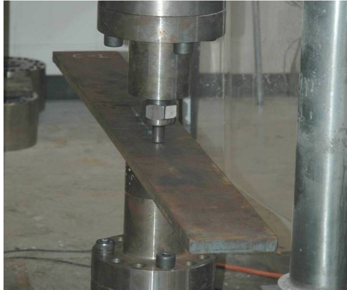
Figure 5-3. View of Hole Punching Operation with Specimen C-1.
