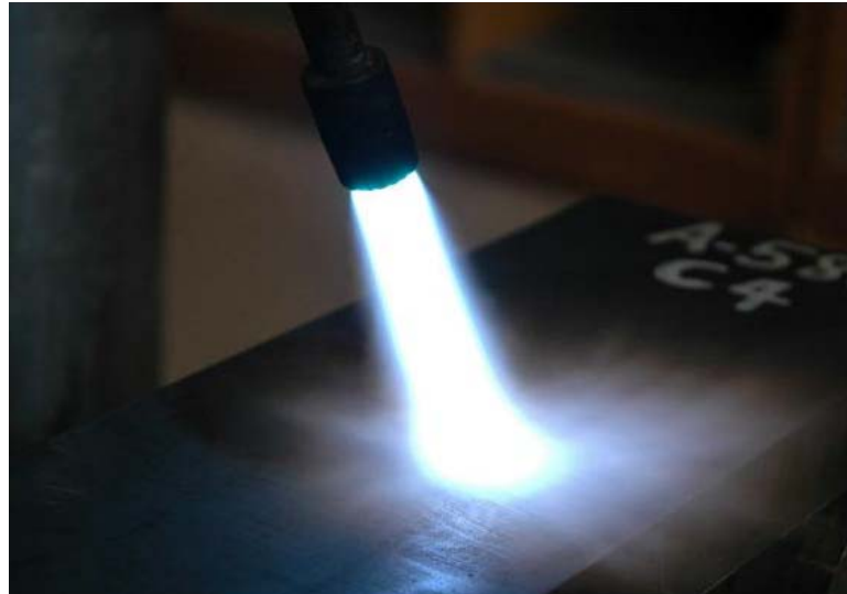
Figure 4-2. Acetylene Torch Heating.
