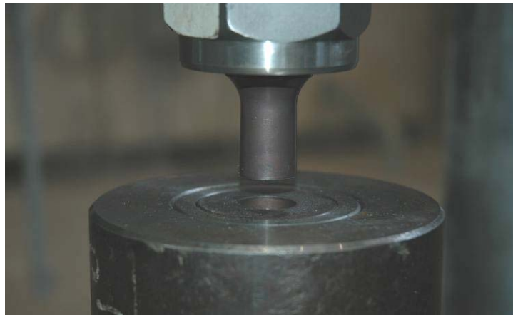
Figure 5-4. Close-Up View of Punch and Die for Specimen Hole Punching.
