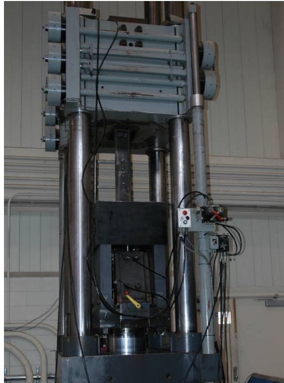
Figure 5-2. 1.5 Million Pound Capacity Load Frame with Non-Loaded Bolted Connection Specimen.
