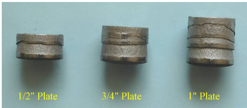
Figure 5-6. Hole Slugs for Three Plate Thicknesses Resulting from Punching Operation.
