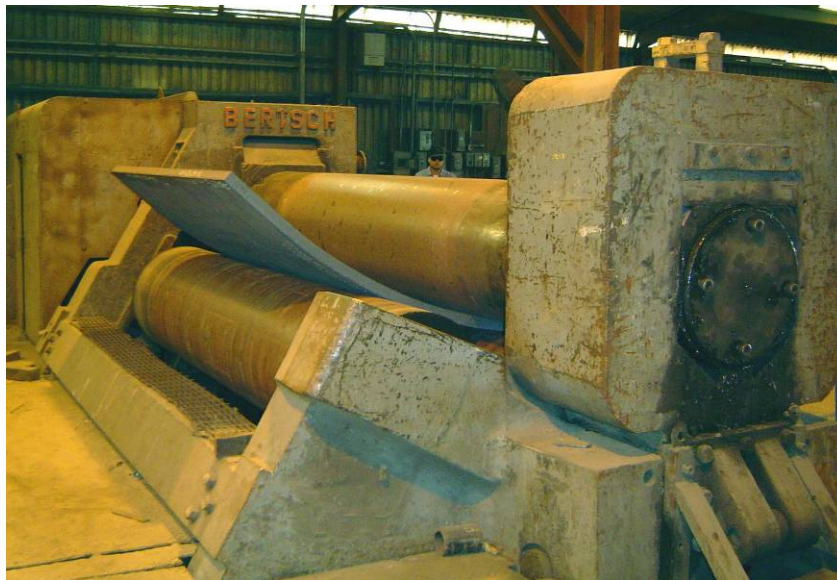
Figure 2-2 View of Pyramid-Type Rolling Bending Equipment for Pressure Vessel Plate.
