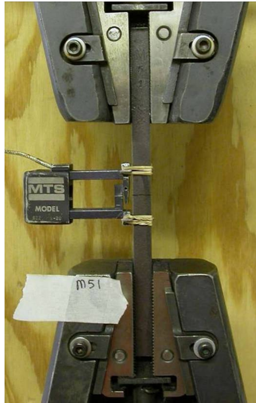
Figure 3-3. View of a Gripped Specimen with Attached Clip Gauge.
