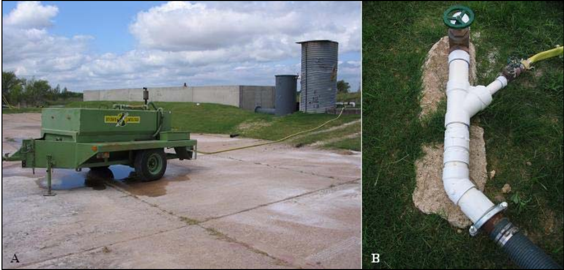
Figure 2.1. A. Hydroseeder for Making Slurry. B. Point of Injection into Main Line.
