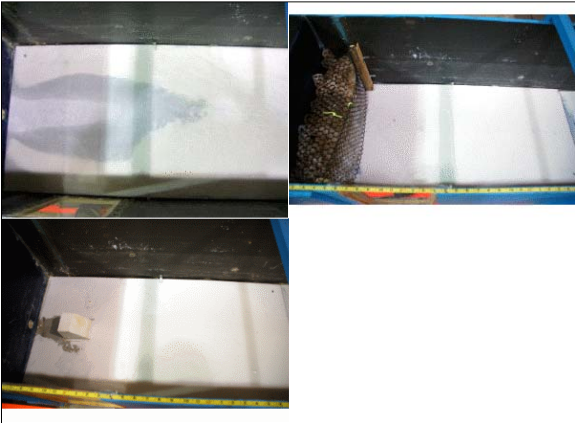
Figure 5.28. Accumulated Particles after Running a Run for the “No Energy Dissipator” Case (Left-Top), “with an Energy Dissipator” Case (Left-Bottom), and “with Flow Straightener” Case (Right-Top).
