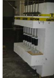
Stressed strand samples (on a concrete reaction frame)
