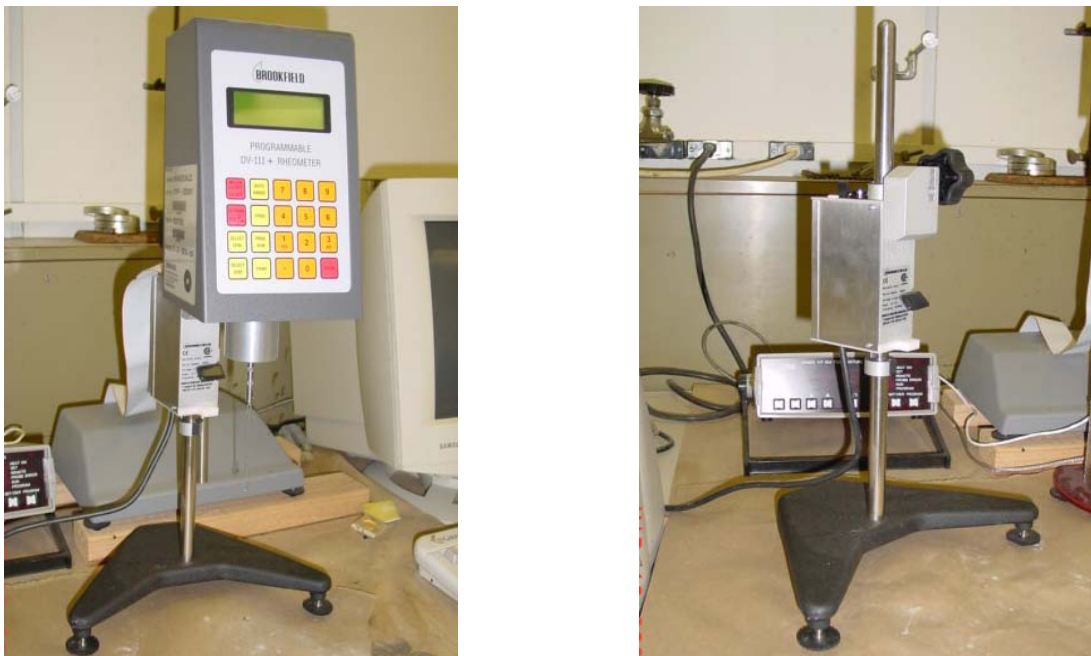
Figure 4-4. Brookfield Rheometer and Helipath™ Stand Used for the Viscosity Test.
