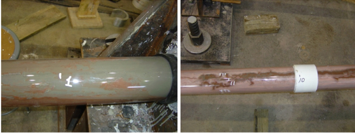
Figure B-13. Repair Grouted Ducts of Specimen PG-C1-1.
