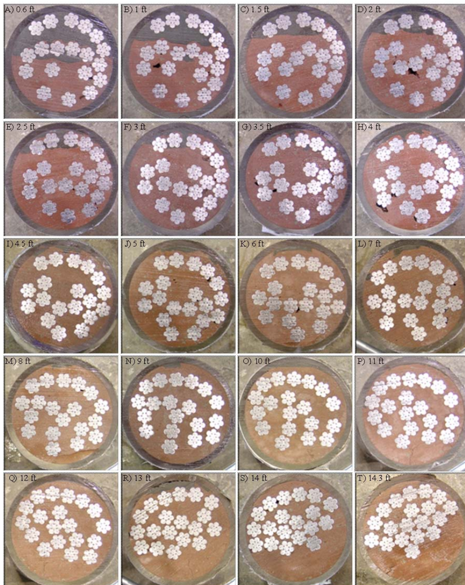
Figure B-35. Cut Sections of Specimen PVG-C1-2 for the Filling Analysis of Repair Grout.
