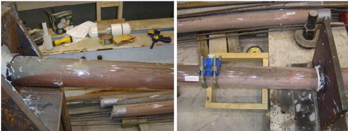
Figure B-31. Repair Grouted Ducts of Specimen PVG-C1-1.
