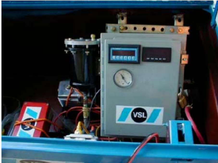
Figure 2-4. Vacuum Control and Grouting Equipment for Voided Tendons (VSL 2002).
