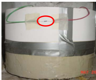
Completely-cast specimen showing the plastic dam and 100 Ω resistor (inside ellipse), and epoxy coated concrete surface
