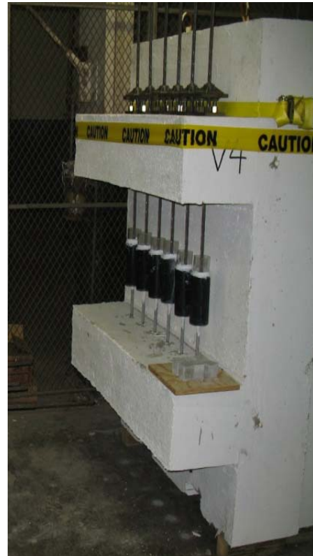
Six stressed OV samples on a concrete reaction frame
