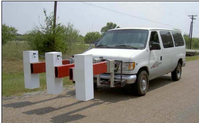
Figure 2.7. Three-Channel GPR System Mounted on Vehicle.
