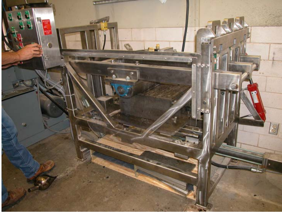
Figure 1.1. Preparation of Laboratory Slabs with Linear Kneading Compactor.
