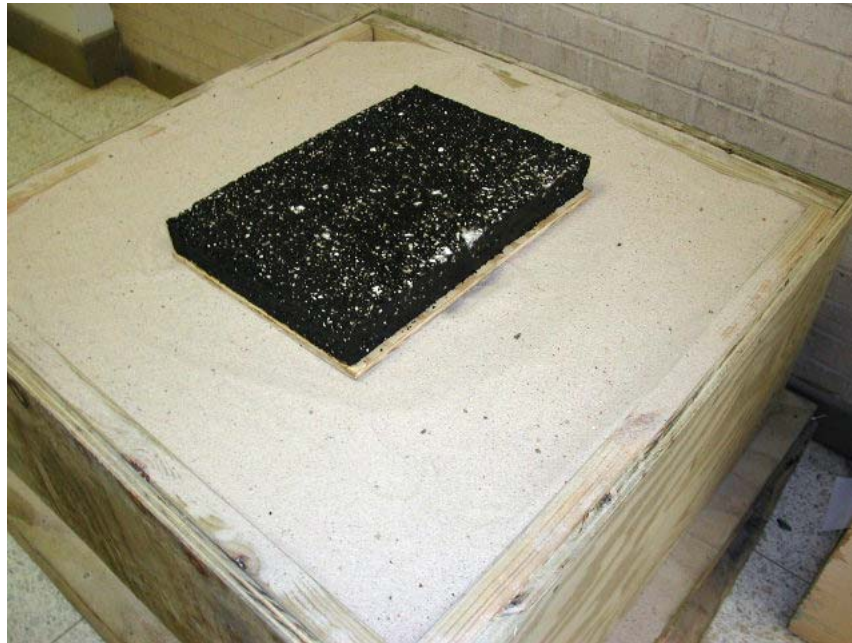
Figure 1.2. Laboratory Slab on Sand Box for Density Testing.
